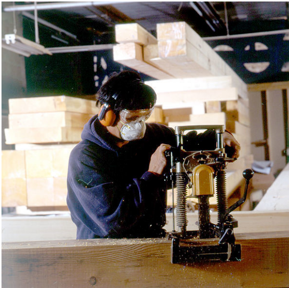
A worker uses a mortising machine to shape timber framing joints
