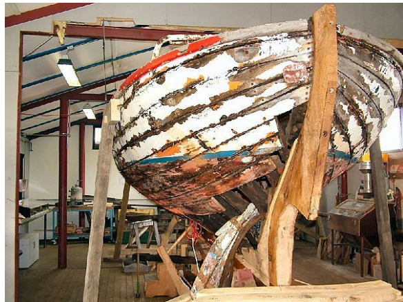
Damaged boat mid-reconstruction; carvel planking partially removed.
