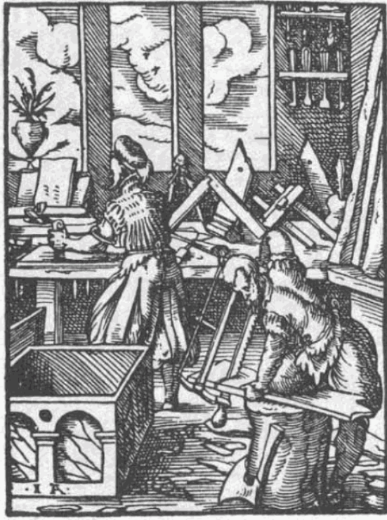
Woodworking shop in Germany in 1568, the worker in front is using a bow saw, the one in the background is planing.
