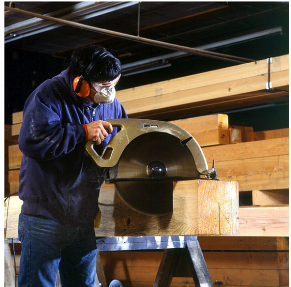
A worker uses a large circular saw to cut joints.
